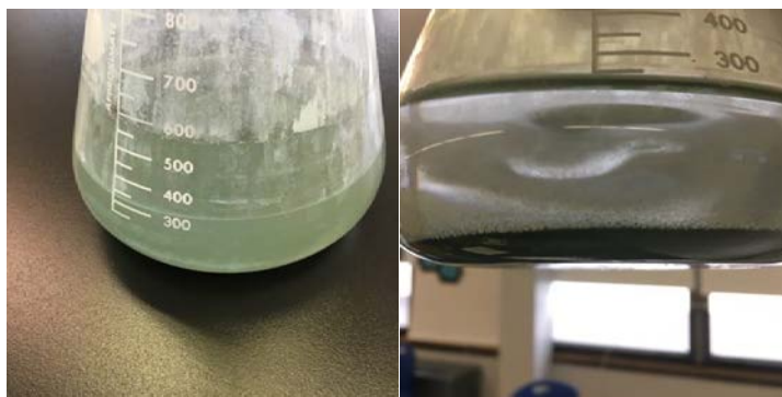
malachite precipitate at bottom of an Erlenmeyer flask
